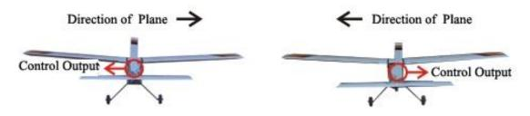
If the compensation direction is not correct, please adjust the Rudder inverse.
