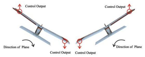
If the compensation direction is not correct, please adjust the Roll inverse.
