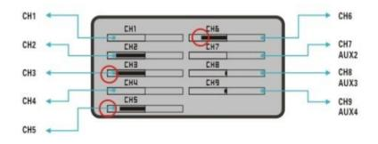
Use CH5 and CH6 to switch flight mode.
