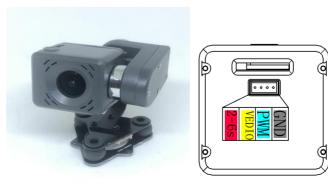
The port behind the camera is: Power, Video, PWM(Not used), Ground (This port supports 7-26V, you can use 2S-6S battery (only for camera!))
