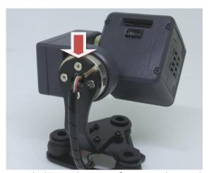
At first, remark the screw hole on the top of motor, then unload the four screws, rotate the aluminum sheet 180 degrees at the back of motor, then re-install it while keeping the motor and the top screw hole position static.
