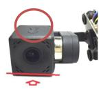
After the calibration is complete, if the blue PWM tilt control line is suspended, the lens will automatically tilt down 15 degrees.
