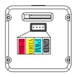
The port behind the camera is: Power, Video, PWM, Ground (This port supports 7-26V, you can use 2S-6S battery (only for camera!))
