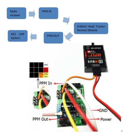
External 433 UHF will supply power for receiving module and radio receiver. The radio PPM signal is connected with PPM input of Arkbird wireless head tracker receiving module; PPM output of Arkbird wireless head tracker receiving module is connected with PPM input of 433 UHF.
