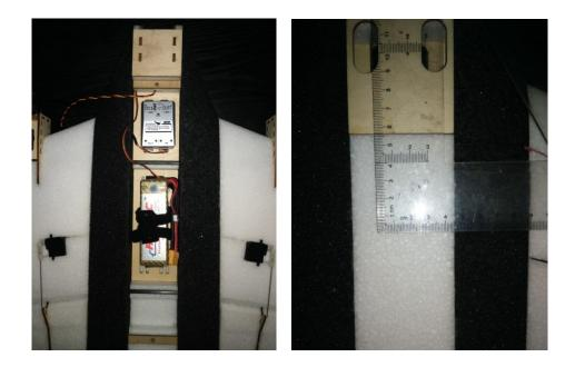
The position of the Flight controller and battery should be as is shown above. It's better to place the VTX somewhere behind battery. We recommend a 4s 2200 to 3000mah battery. A 4s 2200mah battery will look like the one shown above. The position of a 3000mah battery should be about 1cm closer to the nose of the plane
