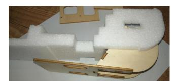
Next, assemble the main fuselage. Follow pictures shown above to stick these parts to the wooden nose. Ordinary foam glue is alright for this.
