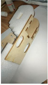
Next, due to the need of VTOL mode, we need to cut away some part of the plastic foam to ensure the upper and lower air holes are under alignment.
