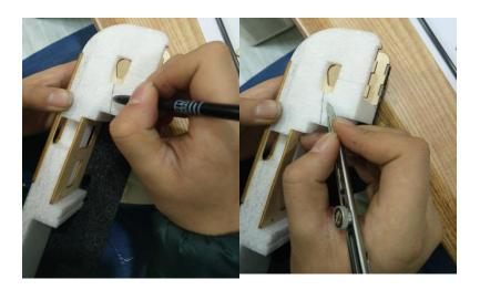
Draw a line on the left part of fuselage like in the picture above, then cut the slot for the wires
