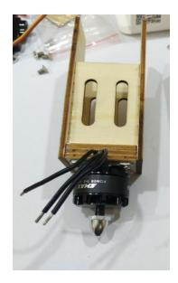
M3 sunk screws, motor mounting base, flat tail tapping screws and shim are packaged in the accessories bag. Please install them on motor mounting base. The finished assembly is as shown above. There are two set, one for each motor.
