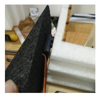
Then, we use the black wing shoulder to stick to the left side and assemble servo as shown above. Place the wires into the slot.
