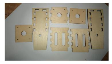
Picking out the parts to assemble motor mounting plate as shown above.
