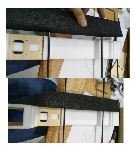
Please present the two black wing shoulders and the two carbon rods as shown above. Use glue (B-7000 recommended) to glue the fuselage and the wing shoulder. Remember to keep the glue away from the carbon rods!
