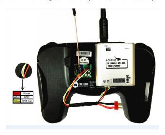
In PPM mode, Radio (Plug T not connected) will supply power for head tracker receiving module and 433Mhz UHF transmitter. PPM signal from radio will be sent to receiving module of head tracker, which will imposes pitch and roll control values to PPM signal Channel 9 and Channel 10. The signal will be sent to 433 UHF.
