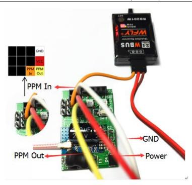
External 433 UHF will supply power for receiving module and radio receiver. The radio PPM signal is connected with PPM input of Arkbird wireless head tracker receiving module; PPM output of Arkbird wireless head tracker receiving module is connected with PPM input of 433 UHF.
