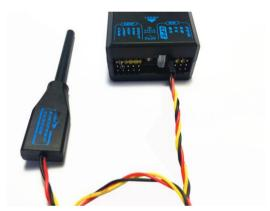
(2) Wiring method of airspeed meter and Arkbird OSD (autopilot 1.0), Please see picture as bellow: (After update Autopilot System with OSD to latest firmware V3.1028, it can be compatible with our airspeed meter.)
