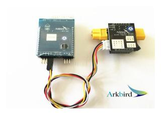
Note: Compare with old Current sensor, it cancel a 2S Battery power supply, reducing weight; add jumper cap and increase the power supply to 1.5A. It can be used on all video tx at the same time.
