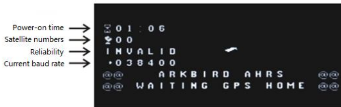
The plane cannot be manipulated when GPS is in the standby interface for a forcible satellite search
